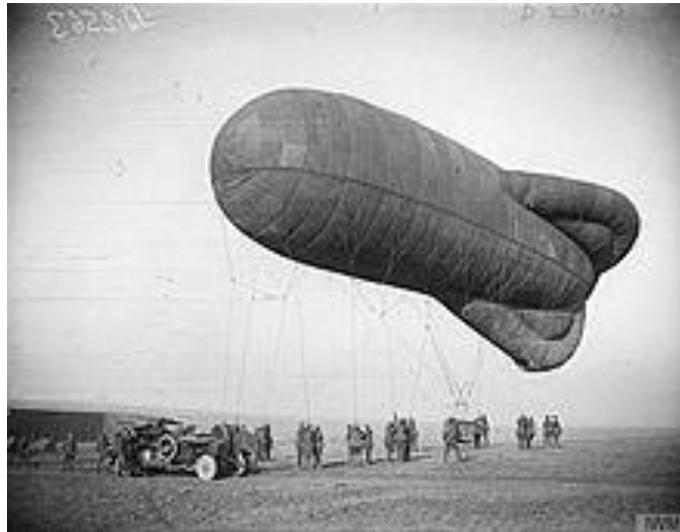
Figure 10: A French Caquot kite balloon. It used wind pressure to inflate one or more stabilising ballonets at the rear, which acted as tail fins. A yoke or harness connected the balloon to the tether and was arranged to aid stability.
