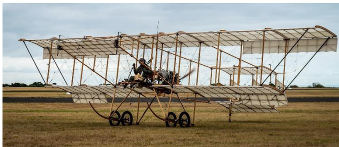
Left -Figure 3: Bristol Boxkite Replica, built at the RAAF Museum and successfully completed flight testing on 11 September 2013. Flown by Air Vice Marshal Mark Skidmore (RAAF retired), a former F-111 pilot and test pilot with the RAAF's ARDU at RAAF Base Edinburgh, the aircraft flew approximately 1000 metres and reached a top speed of about 42 mph. Photograph courtesy RAAF Museum.
