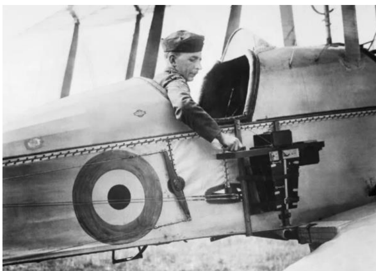
Figure 19: To ensure vertical images, cameras began being mounted on the sides of aircraft. This shows a Type 'C' mounted on a B.E.2c, for operation by the pilot.
